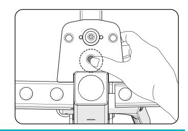
■ Fold Function: Pull up the handle to fold up when not carring bikes. Caution! The handle needs to be placed back to secure the rack.
