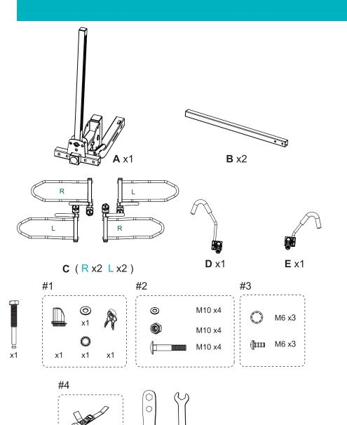
■ Slide the hitch tube (A) into 2" hitch receiver and secure it with Safety Threaded Bolt and kit #1 (External Tooth Lock Washer, Flat Washer and Lock) and lock it.
