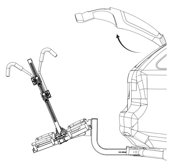
■ The post can fold down laterally by releasing the push buttons.
