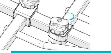
■ Use the kit #3 (Screw and Washer) on the end of the lateral tube to prevent the wheel holders to be slided out.
