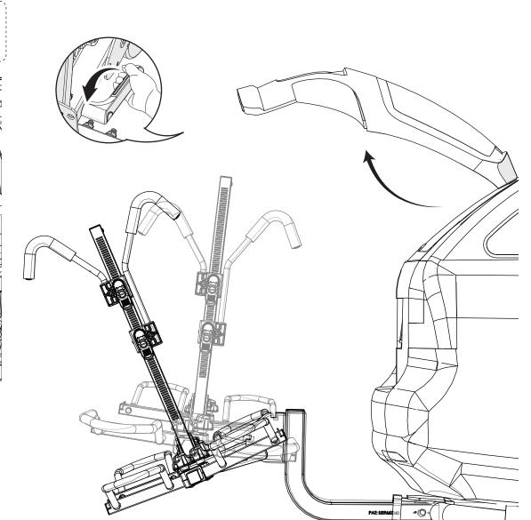
It is not recommended to tilt down the carrier when it carries bikes.
